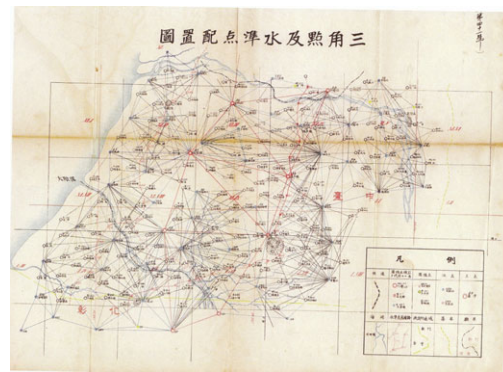
Triangulation points and leveling points
